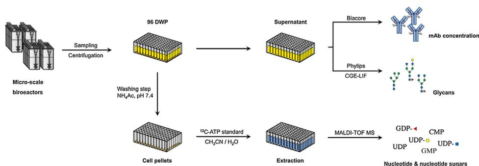
**Fig. 2.** Schematic workflow of the combination of micro-scale bioreactors and analytical techniques. The time-consuming steps such as sampling and extractions procedures are either automated or performed in multi-well plates.
