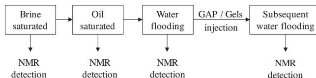
Fig. 2. Flooding procedure of the parallel core flood test.
