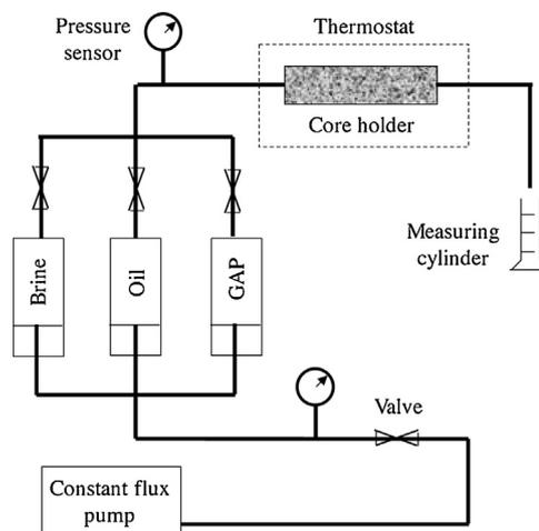
Fig. 1. Schematic diagram of the core flooding system.
