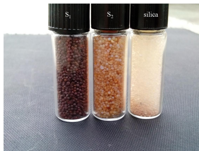
Fig. 1. Low and high iron oxide to silica support weight ratio: \text{S}_1 ( \frac{150\text{ mg Fe}_2\text{O}_3}{\text{g support}} ) and \text{S}_2 ( \frac{12\text{ mg Fe}_2\text{O}_3}{\text{g support}} ) was achieved by manipulating in the amount of silica support.
