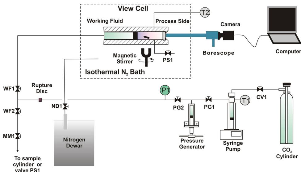
**Fig. 2.** Experimental apparatus used for phase-behavior measurements, including variable-volume view cell, borescope, isothermal N<sub>2</sub> bath, and CO<sub>2</sub> delivery system.
