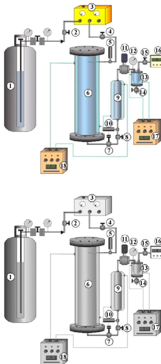
**Fig. 1.** Experimental unit of supercritical fluid process: (1) CO<sub>2</sub> cylinder; (2, 4, 8, 14) flow control valves; (3) gas booster; (5 and 10) pressure transducers; (6) jacketed surge tank; (7) pneumatic control valve; (9) jacketed extraction vessel; (11) forward pressure regulator; (12) manometer; (13) separation vessel; (15) micrometer valve; (16) flow meter; (17 and 18) thermostatic water baths.
