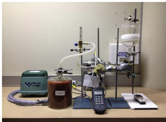
Fig. 2. Photograph of the high inlet gas temperature bubble column sterilization apparatus.
