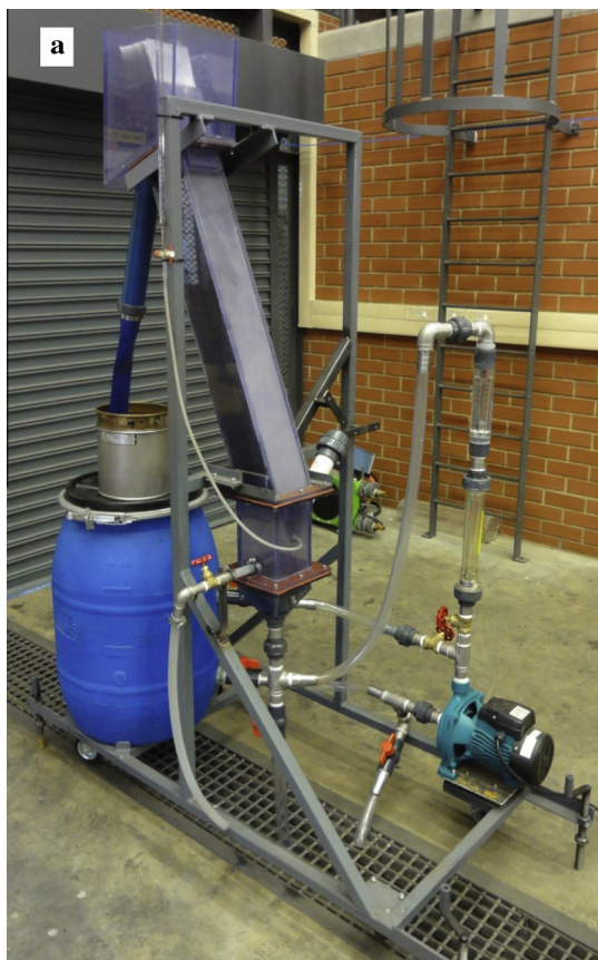
Fig. 1. Photograph (a) and schematic (b) of the experimental laboratory reflux classifier.
