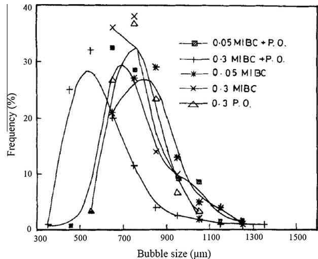
Fig. 3. BSD generated by porous plate with frother (Biswal et al., 1994).
