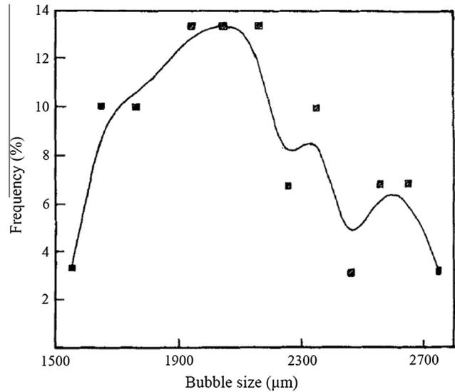
Fig. 2. BSD generated by porous plate without frother (Biswal et al., 1994).
