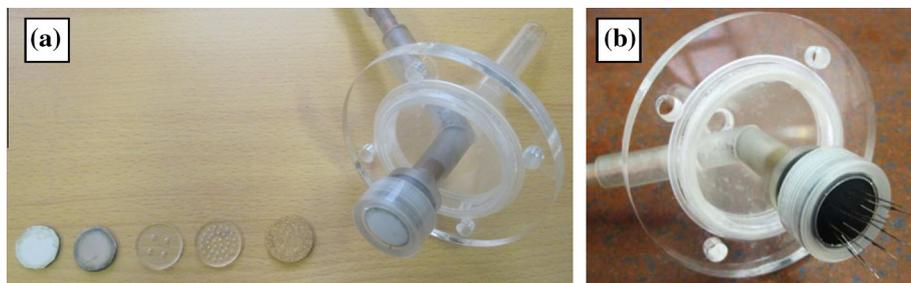
Fig. 1. (a) Sparger with the ability of changing orifice and porous plates, (b) plate of needles to generate uniform size of small bubbles.
