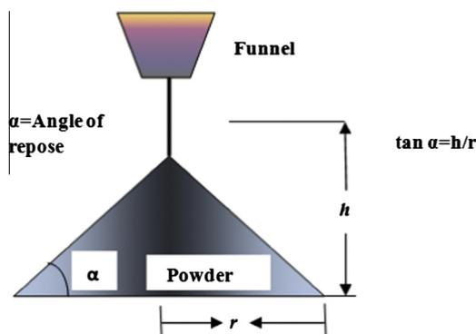
Fig. 1. Carney funnel used in measuring the angle of repose of particles less than 5 mm size, adapted from Datta (2012).
