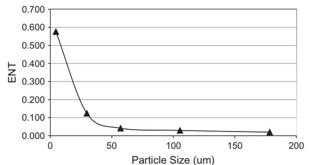
Fig. 1. Example of the decay of entrainment with particle size.
