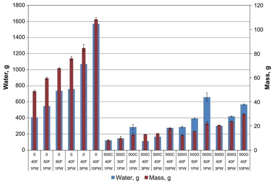
**Fig. 1.** Final mass and water recovered for batch flotation tests conducted under 0 g/t and 500 g/t guar (G) and CMC (C) while increasing ionic strength (PW) or increasing frother dosage (F).
