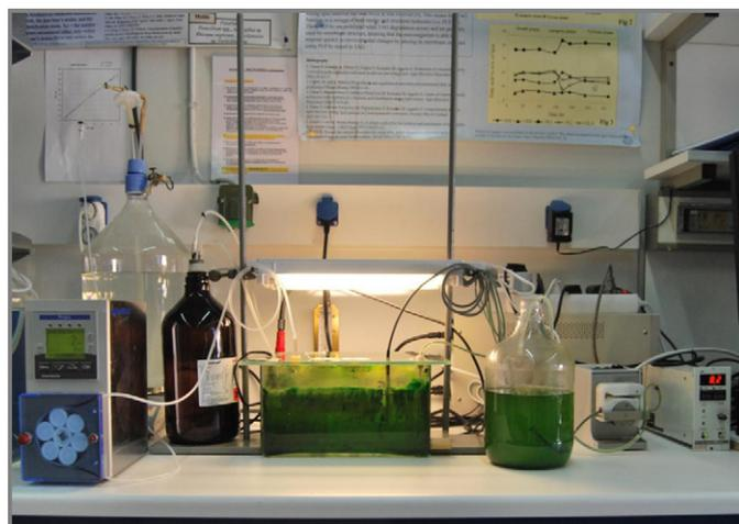
**Fig. 1.** The open pond simulating photobioreactor designed and used for the current study. Characteristics: depth, 15 cm; surface area, 590 cm<sup>2</sup>; total volume, 8.7 L; working volume 5 L; agitation was achieved by a circulator; moisture air supplied at 0.5 vvm; light illumination, 120 μE m<sup>-2</sup> s<sup>-1</sup>.
