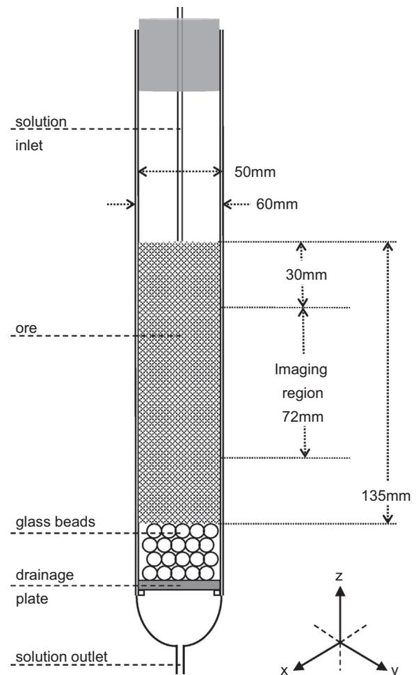
**Fig. 1.** Schematic of the leaching column with the ore bed and imaging region heights indicated.
