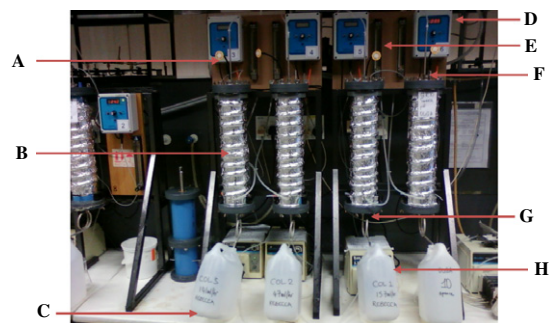
Fig. 2. Heap leach columns (A – Air outlet, B – Column, C – PLS collection vessel, D – Temperature sensor, E – Rotameter, F – Inlet feed point, G – Air inlet, H – Pump).
