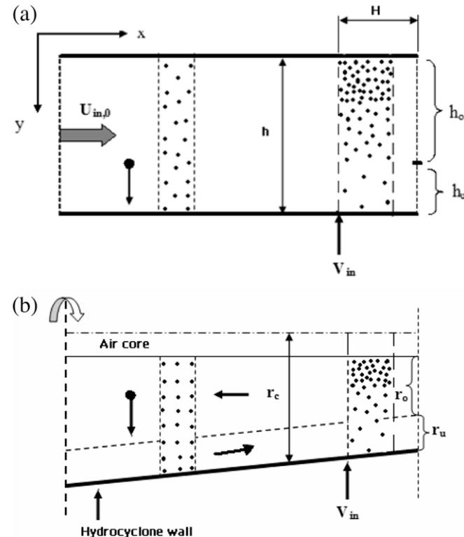
Fig. 1. Separation model of: (a) cross flow classifier, (b) hydrocyclone.
