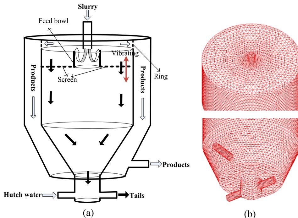
Fig. 1. (a) Schematic representation of in-line pressure jig and (b) the mesh used in CFD.
