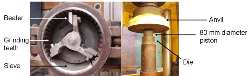
Fig. 1. (Left). Interior chamber of the hammer mill; (Right) piston–die compression unit.
