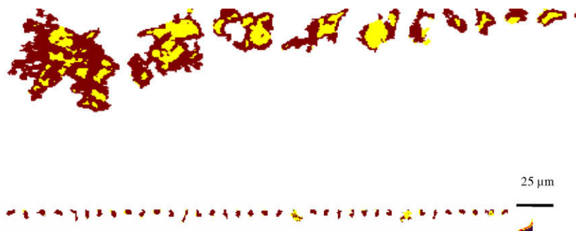
Fig. 2. False-colored digital images of pyrite grains (light, centers) with arsenian rims (darker) from the Chukar Forrwall deposit, Nevada. Sub-micron-sized gold occurs in arsenian-pyrite rims within Carlin-type systems. Identification of arsenian-pyrite can be used as a proxy for gold mineralization.
