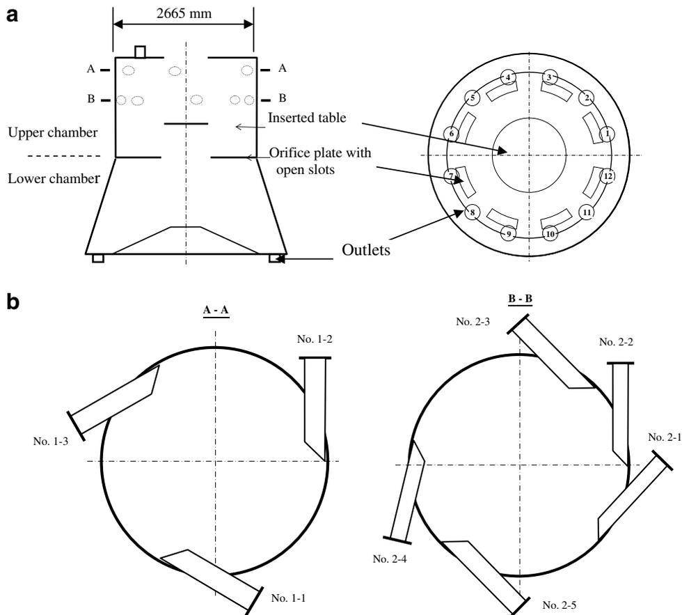
Fig. 1. Schematic illustration of the distributor considered: (a) side and plan view of geometry, internal structure and numbering of outlets; and (b) orientation and numbering of water inlets for both level.
