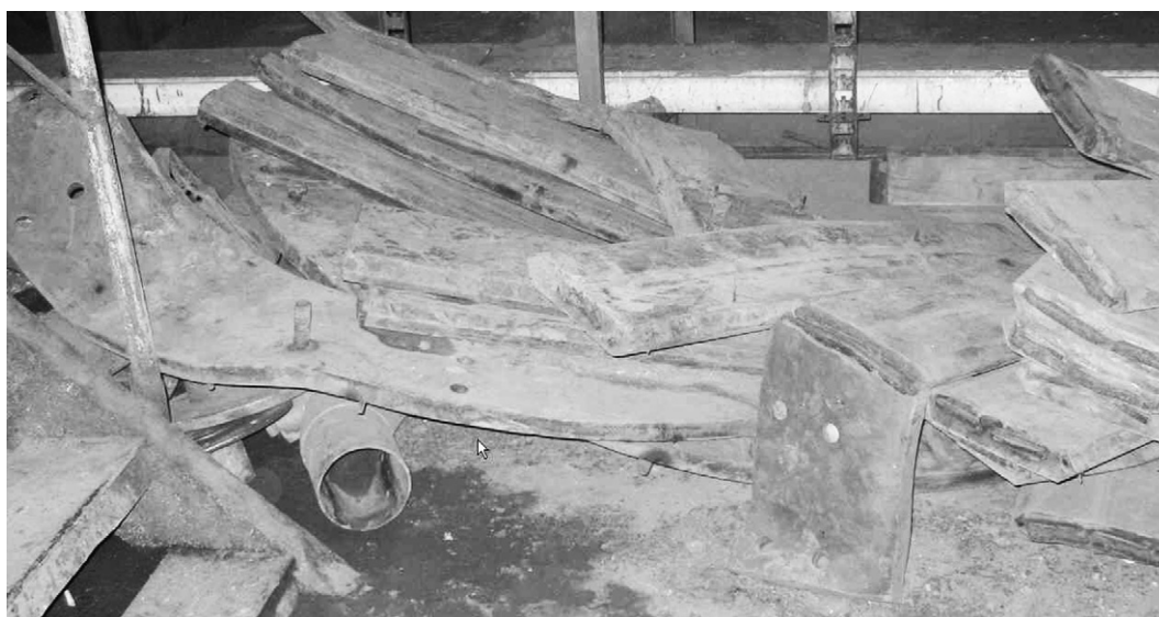
Fig. 2. Pirate flotation cell mixer spare parts after two weeks of use.
