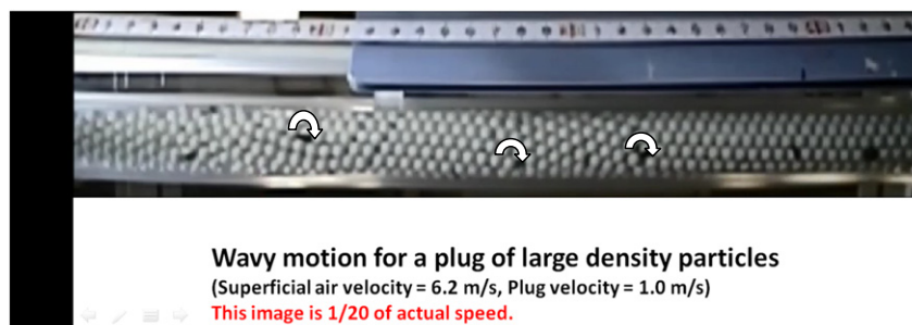
Fig. 2. Rotating particles in dense phase plug conveying.
