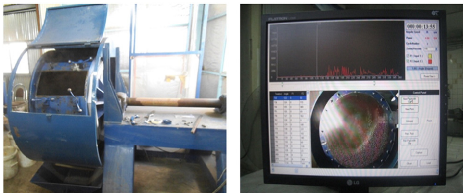
Fig. 1. Schematic of the experimental pilot mill and the monitoring of the device.
