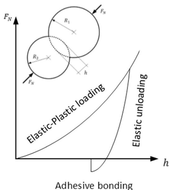
Fig. 1. Sketch of a representative force–displacement relationship pertinent to simulation of powder compaction.
