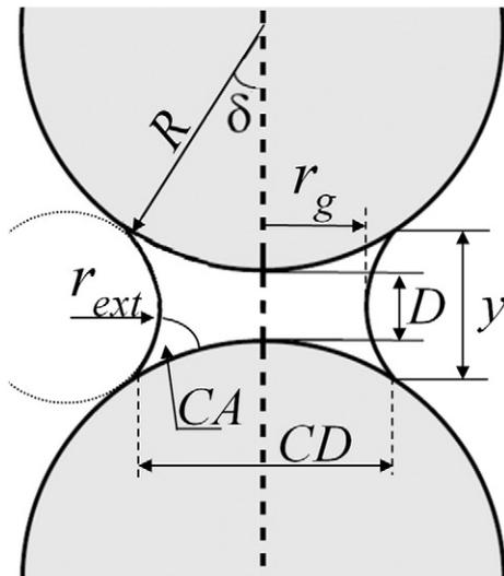
Fig. 1. Liquid bridge between two spheres.
