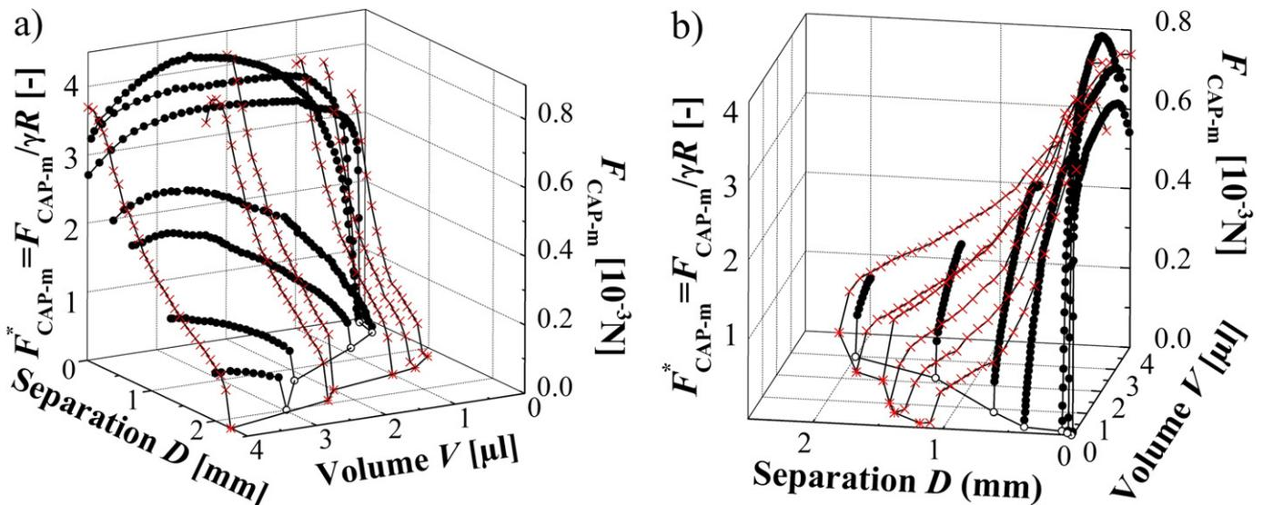
Fig. 2. Two views of total capillary force evolution measured during evaporation tests at constant separations (bullets) and during extension tests at a specific constant volume, starting from zero separation (crosses). Notable is the discrepancy between the force values from the two types of a constant separation or volume cross-sections for the two tests especially marked at smaller liquid volumes and smaller separations.
