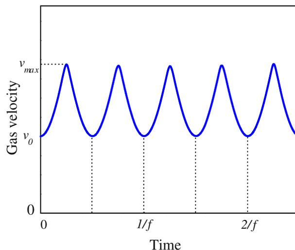
Fig. 2. Waveform of pulsing airflow.
