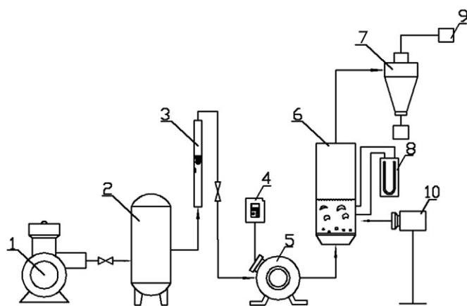
Fig. 1. Schematic of experimental system: 1 – blower, 2 – tank, 3 – flow counter, 4 – inverter, 5 – ball valve, 6 – fluidized bed, 7 – cyclone dust collector, 8 – U-tube manometer, 9 – bag filter, 10 – high-speed camera.
