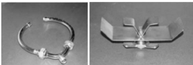
Fig. 1. Perforated dispersion ring (left) and rebound nozzle (right).
