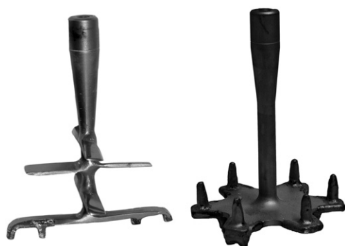
Fig. 1. High-shear mixing tools for the Eirich-type high-shear mixer. Star agitator (left); pin agitator (right).
