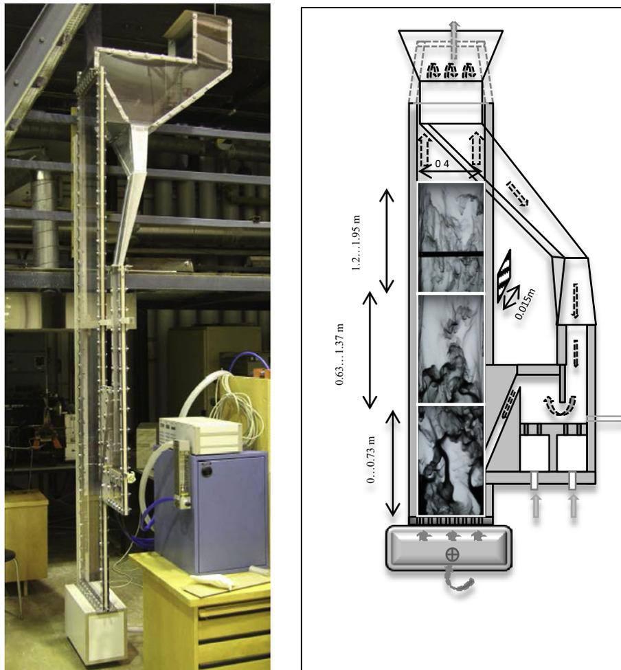
Fig. 1. Left: Photograph of the lab-scale CFB. Right: Functional diagram of the CFB along with experimental images from heights  $z = 0.00\text{--}0.73 \text{ m}$ ,  $0.63\text{--}1.40 \text{ m}$  and  $1.40\text{--}2.20 \text{ m}$ .
