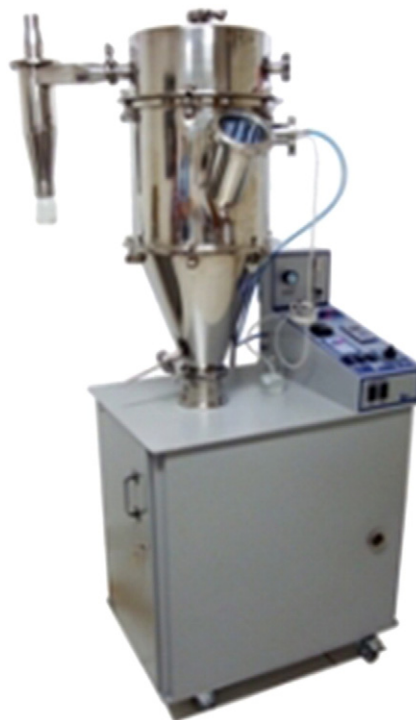
Fig. 1. Fluidized bed FBD 3.0 with 3-kg capacity (reproduced with permission of Labmaq do Brasil Ltda, Ribeirão Preto, SP, Brazil).
