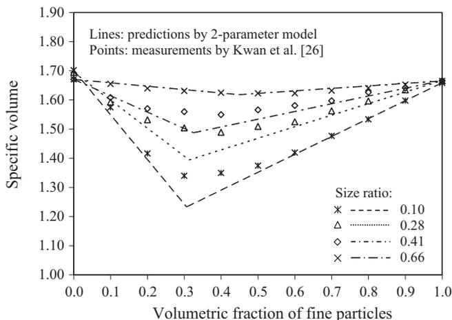
Fig. 1. Variation of specific volume with volumetric fractions.
