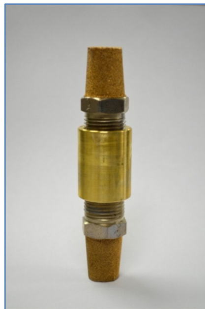
Fig. 2. Photograph of the powder-holder piece composed of two opposite filters of sintered porous metal (filter elements available in pore sizes ranging from 0.5 to 140 \mu\text{m} ).
