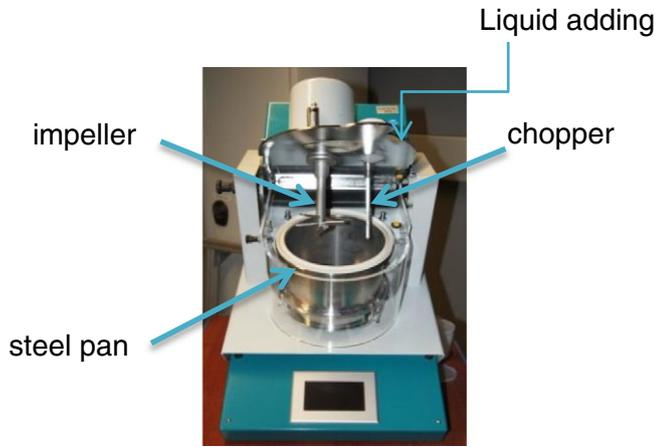
Fig. 1. Eirich high-intensity granulator (impeller diameter 7.7 cm, steel pan diameter 16.5 cm).
