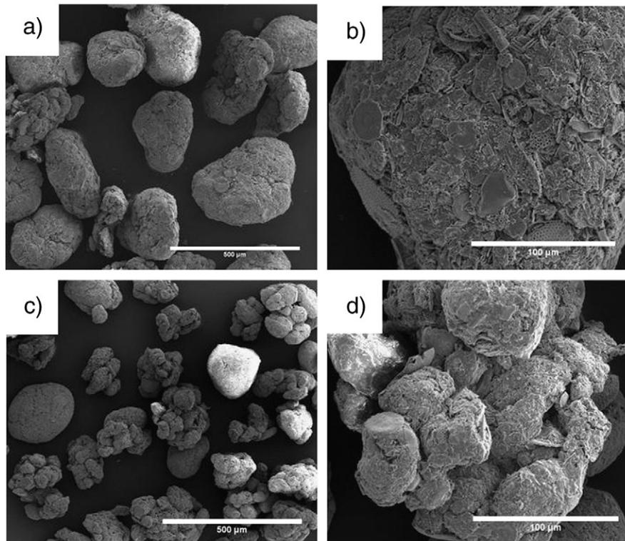
Fig. 2. Top view SEM images of sintered granulates fabricated under different pan rotation speeds: (a and b) granulates fabricated at pan rotation speed 85 rpm, (c and d) granulates fabricated at pan rotation speed 170 rpm. The scale bars in panels a and c are 500 μm, in b and d are 100 μm.
