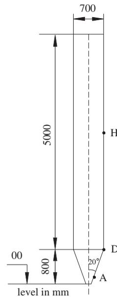
Fig. 1. Configuration of the Danish model silo: a cylindrical bin with a conical hopper.
