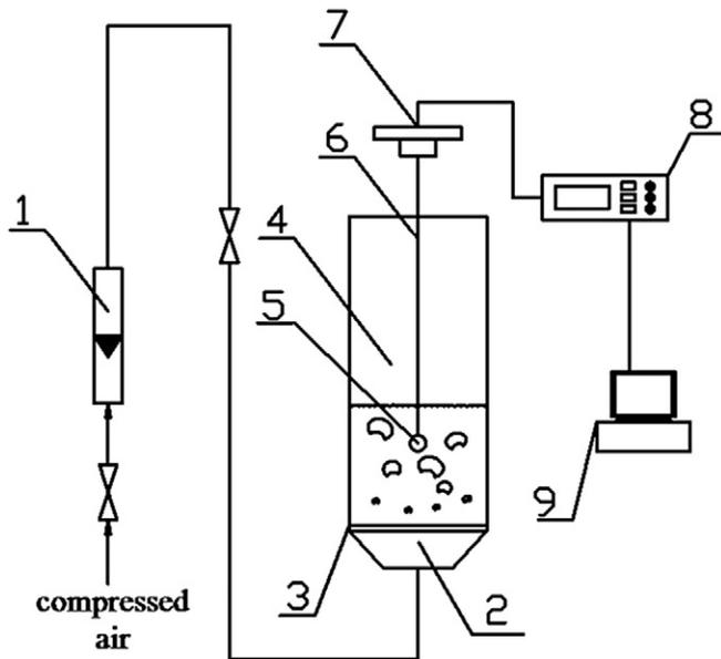
Fig. 1. Force measurement system of the large coal particle in a dense medium gas–solid fluidized bed. [1. gas flow meter; 2. air chamber; 3. gas distributor; 4. gas–solid fluidized bed; 5. large coal particle; 6. flexible line; 7. force sensor; 8. signal converter; 9. data receiver and monitor].
