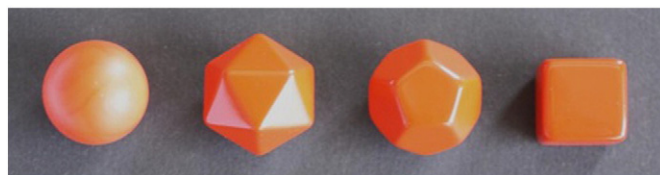
Fig. 1. Test particles from left to right: sphere, icosahedron, dodecahedron, hexahedron.
