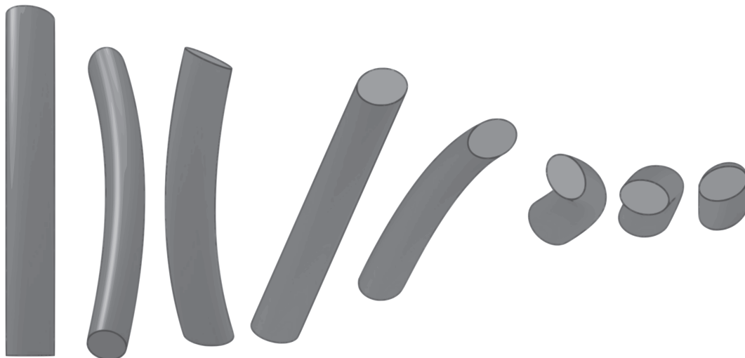
Fig. 1. The effect of three dimensional irregular shape on the two dimensional size and shape measurement.
