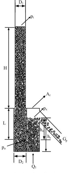
Fig. 2. Schematic diagram of loop-seal.
