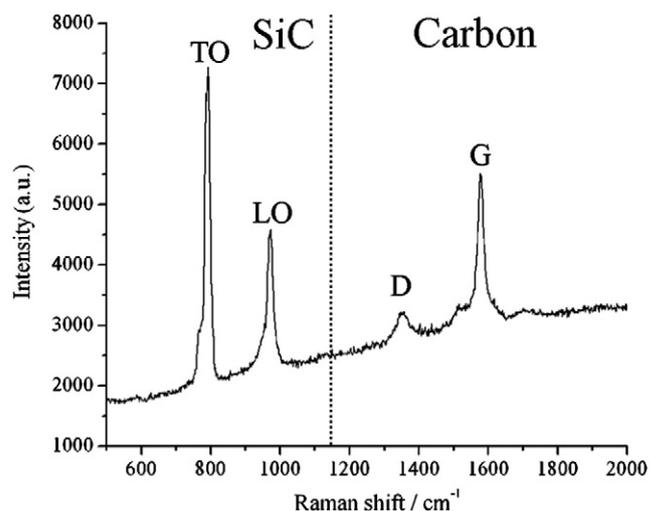
Fig. 2. Raman spectra of the synthesized silicon carbide powders.
