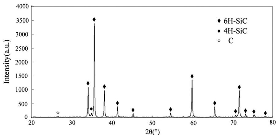
Fig. 1. X-ray diffraction pattern of the synthesized silicon carbide powders.
