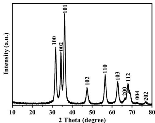
Fig. 2. XRD patterns of the prepared ZnO.
