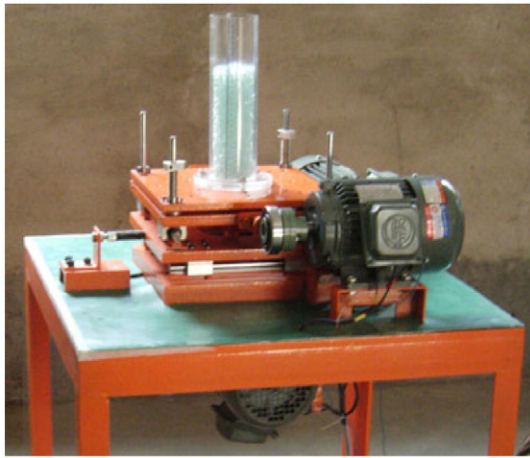
Fig. 1. (a) Physical setup; and (b) schematic view of the vibration setup. 1, container; 2, 5 and 7, guide rail at three directions; 3, electromotor; 4 and 6, vibrating desk along X and Y directions; 8, shaft along the Z axis; 9–11, frequency control of vibration at three directions; 12, transducer; and 13, transmission and amplitude control device.
