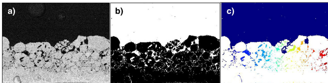
Fig. 1. Steps for image analysis a) initial image, b) binarised image (cracks are in white), c) detection of cracks (each crack is in different colour). (For interpretation of the references to colour in this figure legend, the reader is referred to the web version of this article.)
