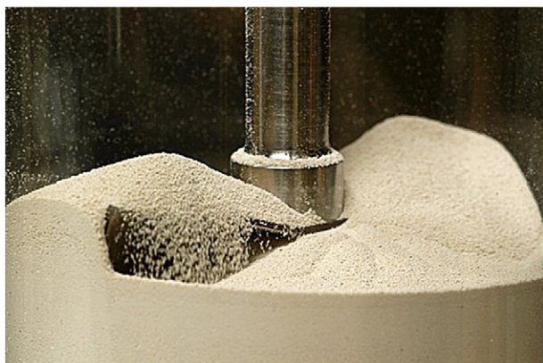
Fig. 1. Photo of the end of a conditioning traverse showing the blade moving upwards out of the powder.
