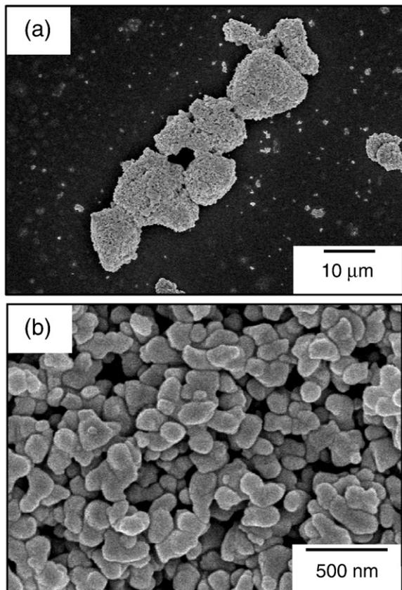
Fig. 2. SEM images of the  $\alpha$ -alumina particles observed at (a) = low magnification and (b) = high magnification.
