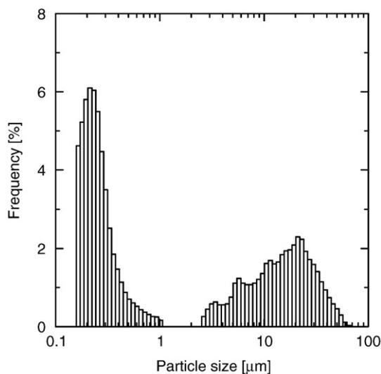
Fig. 3. Particle size distribution of the suspension before mesh treatment.
