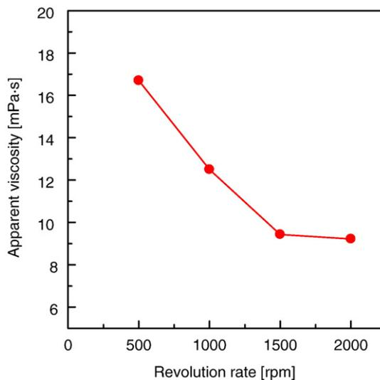
Fig. 4. Apparent viscosity of the suspension after mesh treatment as a function of the revolution rate.
