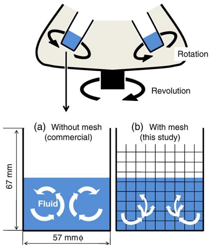
Fig. 1. Schematic model of the instrument for particle dispersion.
