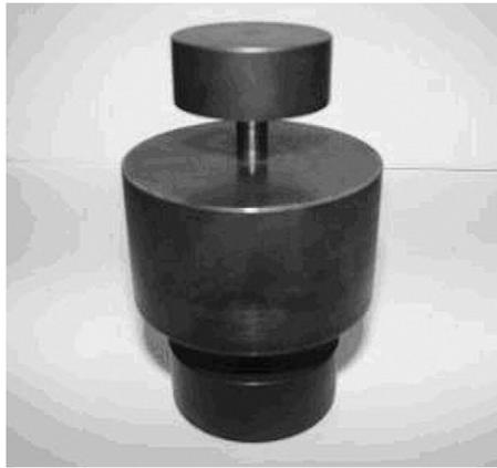
Fig. 2. Matrix to obtain the samples.
