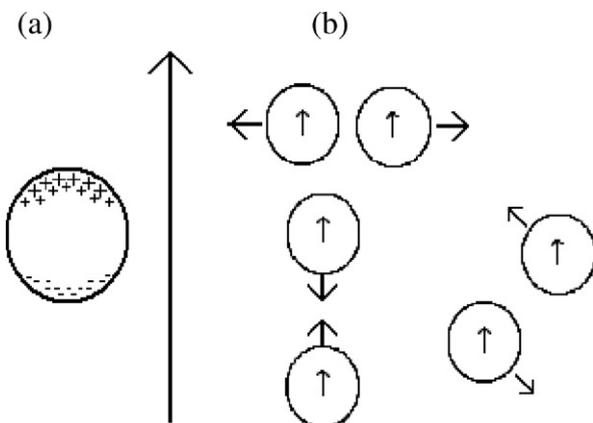
Fig. 1. (a) Maxwell–Wagner polarization of spherical particles, showing the migration of charge to the poles of the particle. (b) The direction of the electric-field induced interparticle force for various particle orientations.
