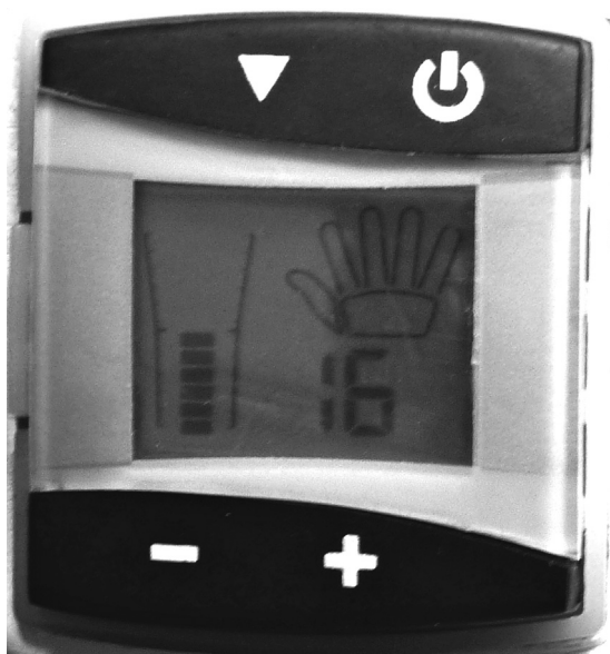
Fig. 1. The display of the computer with the visual scale and the sensitivity number.
