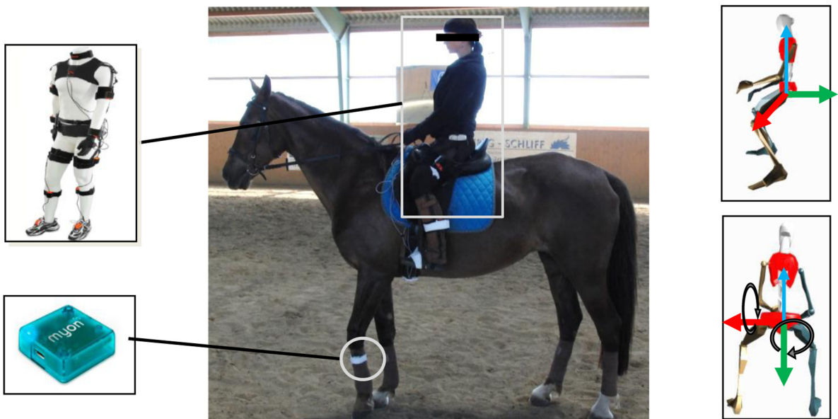
Fig. 1. Experimental setup: rider (MVN suit) and horse (acceleration sensor on the cannon bone) with the applied measurement systems: Rotation axes of the riders' segments are shown as arrows: red arrows indicating roll angles; green arrows indicating pitch angles [22].
