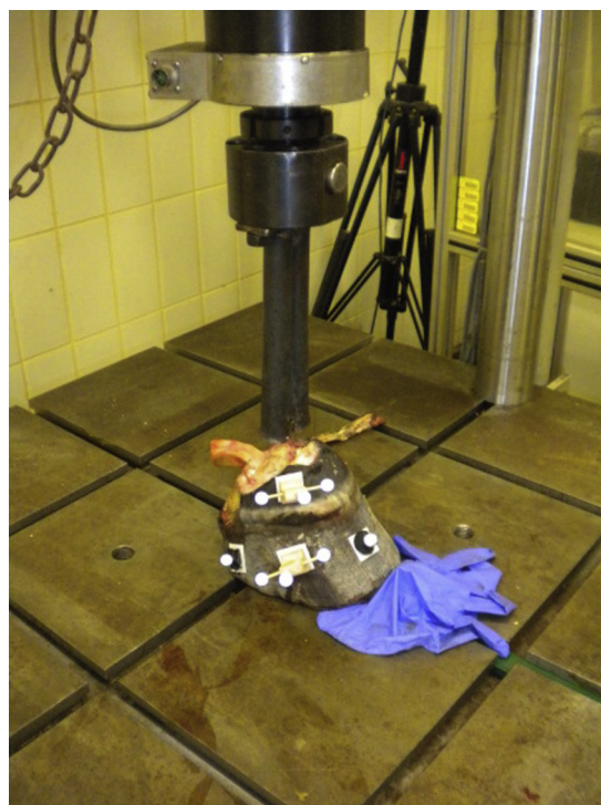
Fig. 1. Specimen (horse 2, right forelimb) in the material testing machine. Tripods with the reflective markers attached to the lateral sides of the second and third phalanx. The base of the third phalanx tripod is covering the defect in the lateral hoof wall. In addition, one marker on the heel and one dorsal on the hoof wall are visible. The marker on the opposite heel is obscured. The glove in front of the dorsal hoof wall is covering an adjusting screw that would have caused reflection errors during kinematic measurement. The adjusting screw was necessary to keep the specimen in its position during load measurement.
