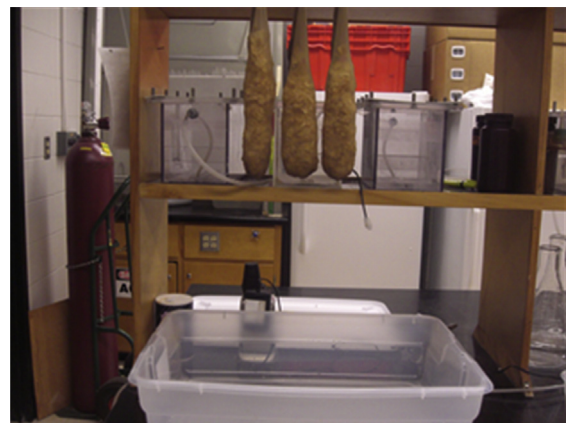
Fig. 2. Draining off excess water from bedding material after immersing for predetermined time.
