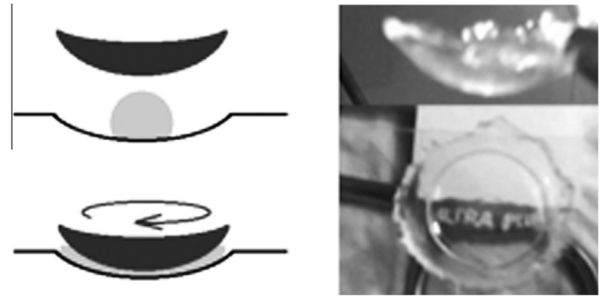
Fig. 1. Transparent collagen matrix at 90 mg/mL. Left side illustrates the molding of the collagen dense solution prior setting into ammonia vapors. Right side shows the collagen matrix after fibrillogenesis.
